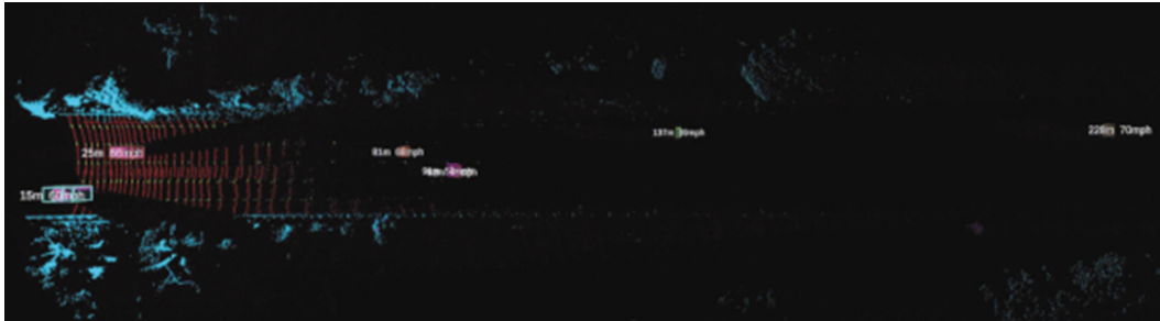
Our perception software detecting, tracking, and classifying vehicles, lanes, objects, and drivable free-space, up to 250 meter away, in real-time.
