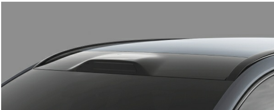
Our Iris lidar sensor integrated into Volvo SPA2 platform with expected production in 2022
